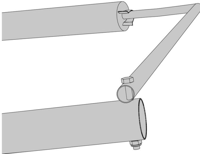
Illustration 3 – Model C wing tip tube correctly bolted to top of trailing edge, creating a built-in washout of 0.9 degrees. \*
