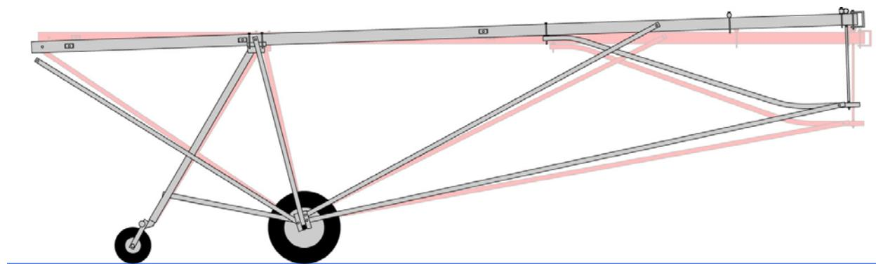
Illustration 4 – Comparison between level boom (shaded red) and negative 2 degree down angle boom.
